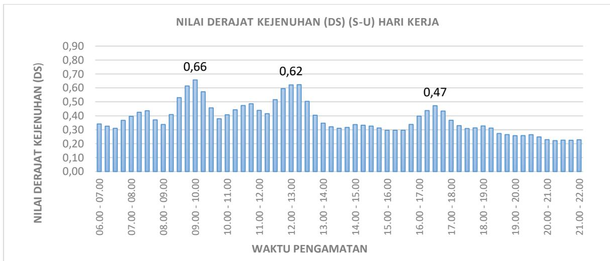
**Figure 7. Graph of Degree of Saturation (DS) on the Medan Pematang Siantar Road Section**
