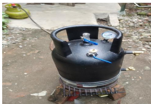
Figure 1. Modified 12kg LPG cylinder boiler design
