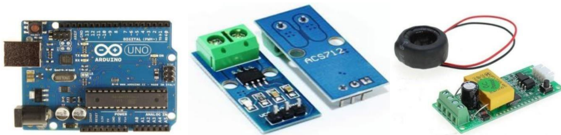
Figure 3. Arduino Uno, Current Sensor and Voltage Sensor
